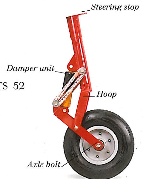
NOSE-GEAR OF A MODERN LIGHT AIRCRAFT
